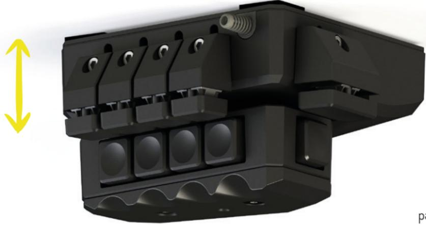
To do so, loosen the fixing screw of the selected secondary key with the enclosed Allen key (3 mm) by a maximum of two turns and position it by carefully moving it to the desired height. Then tighten the fixing screw again. In this way, you can adjust all front secondary keys individually.
